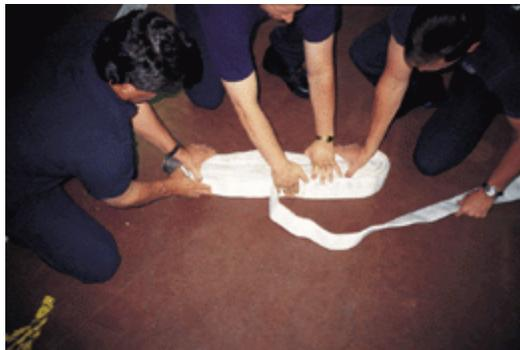
Each time the hose reaches the point near the male coupling, stagger the folds, one long and one short, similar to an accordion-type hose load in the main hose bed of some pumpers. This keeps it neat and compact and maximizes space.
