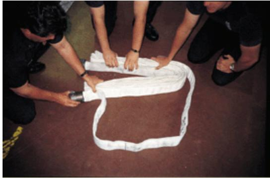
Place the female coupling on the side of the horseshoe opposite that of the male coupling and just past the hose folds. This helps to balance the hose pack and distribute the weight more evenly.
