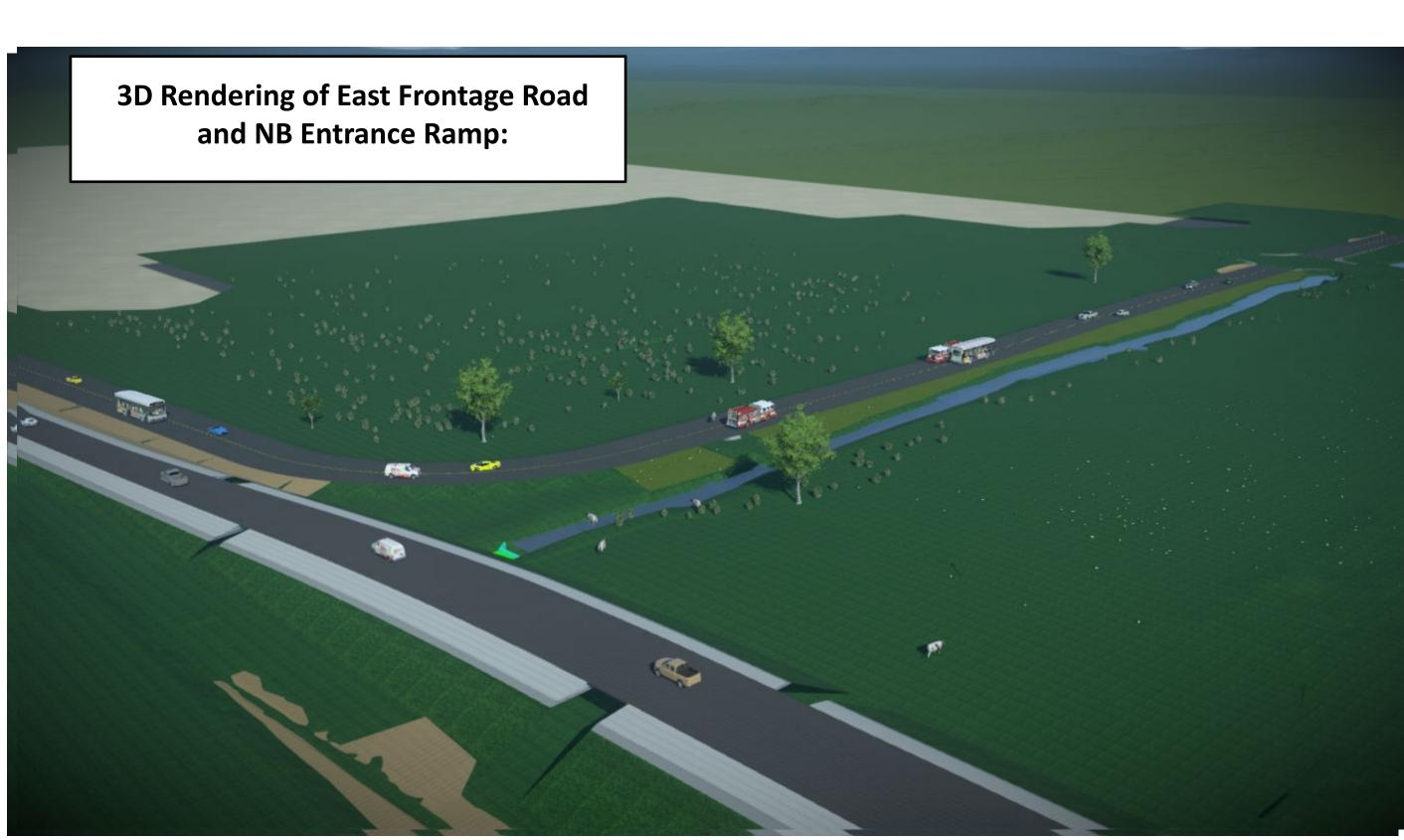
**Create 3D Model: Combining these** elements allows for the creation of 3D models which can be used to see what the road will be like once constructed. 3D models provide roadway quantities which can be used for estimates.
