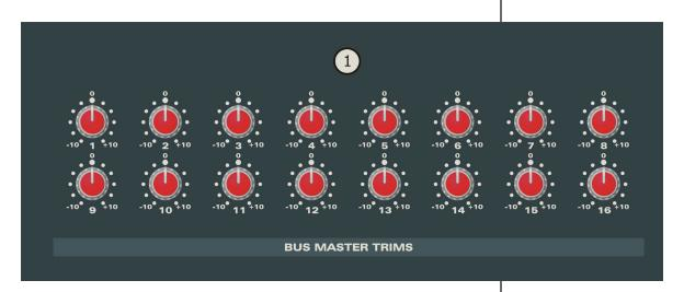
BUS MASTER TRIM controls the overall level of a bus output. The BUS MASER TRIMS are the final stage of level control over the signals routed to the bus outputs. Each bus output has a trim with a range of  $\pm 10 dB$ .
