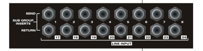
This panel carries the connectors for the sub-group insert points. There are 8 sub-groups and each insert point has a send output and a return input.
