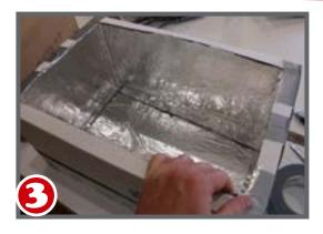
Set the inner box on top of the copy paper box and trace a line around it onto the folded lip. Cut along the traced line to form a hole that fits the inner box.
