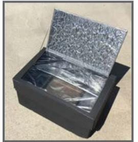
to the lid to direct more sunlight into your oven. Make additional wire props to hold the reflector flaps open.
