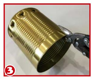
resulting flap up to create a large vent. Use caution bending the flap. The sides of the metal are very sharp.
