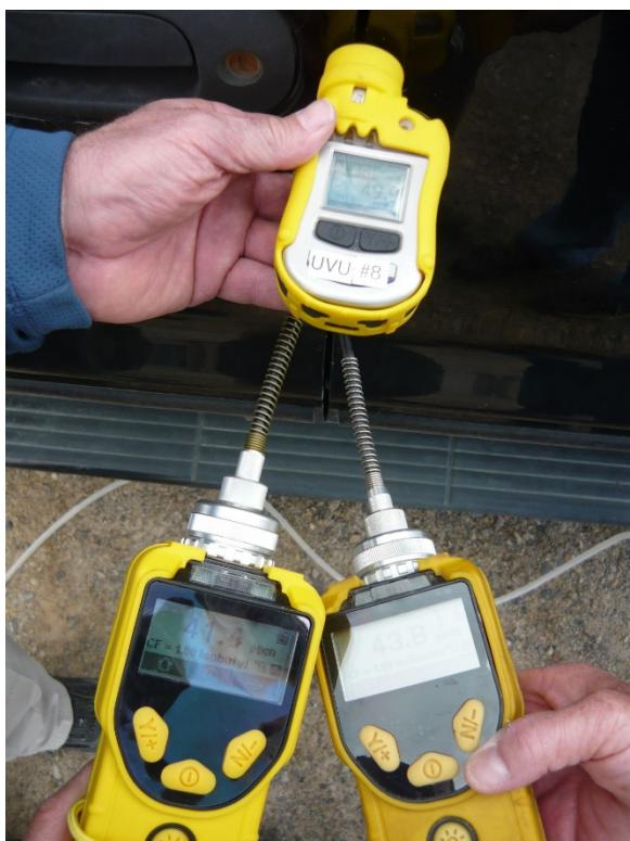
Figure 8. Field calibration of the RAE Systems PID.
