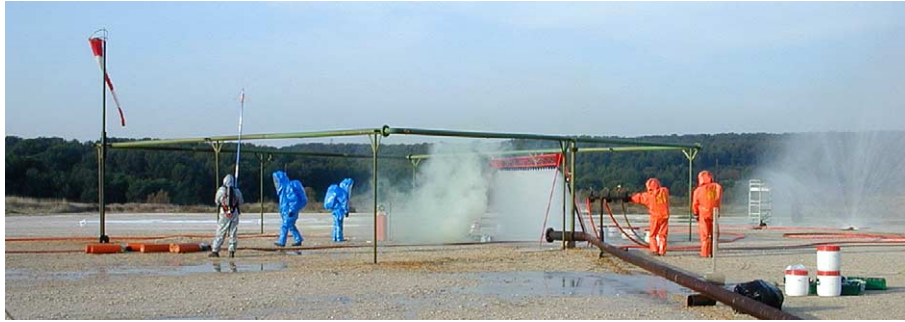
Fig. 2. Forced dispersion, field test, R_M=10.7 .
