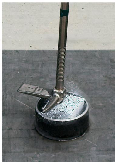
**Fig. 5.** Moment of impact of a Halligan tool dropped on a conditioned asphalt sample.
