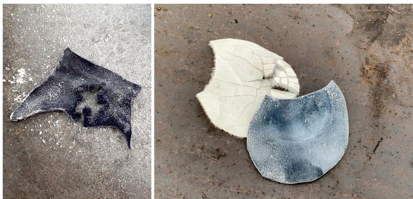
Fig. 7. Post-impact: contaminated glove (a) and new glove (b).
