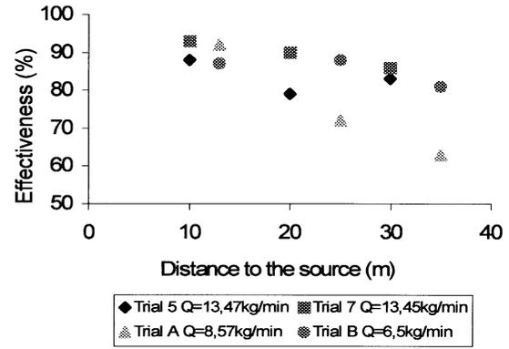
Fig. 4. Comparison of effectiveness behind the curtain for different release rates of ammonia.
