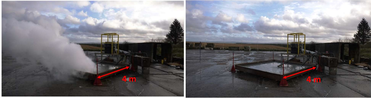
Figure 8: RS-1F unpressurized/cold ammonia spill on water in bund with initial puff discharge for 18 seconds (left) and aqua ammonia pool after release (right)
