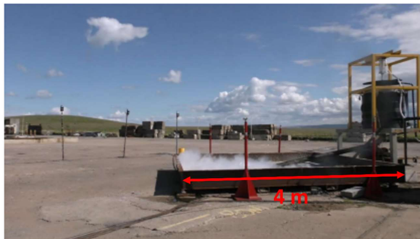
Figure 7: RS-1C unpressurized/cold ammonia spill on concrete in bund
