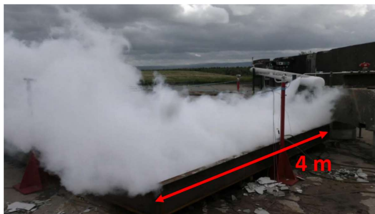
Figure 11: RS-3F refrigerated, pressurized ammonia release
