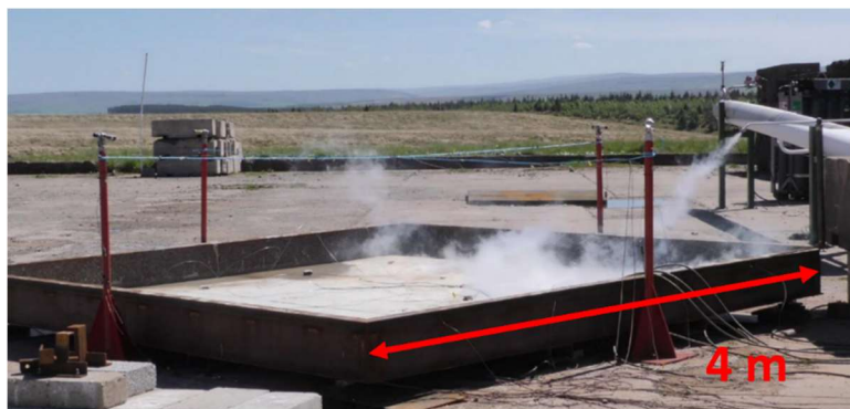
Figure 10: RS-3A refrigerated, pressurized ammonia release
