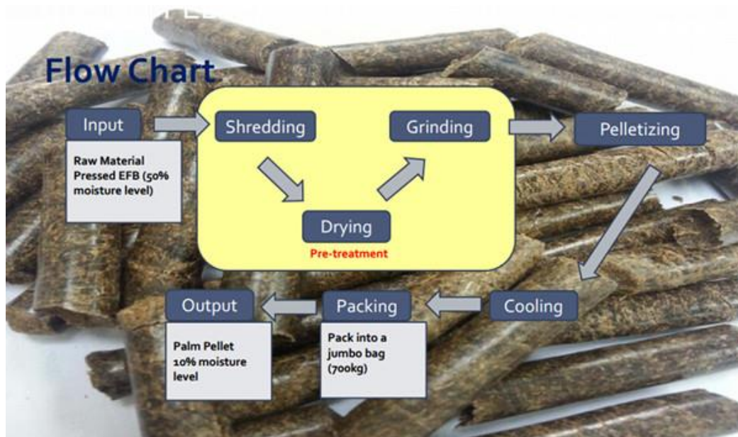
Figure 4: EPFB Pellet Making Process
