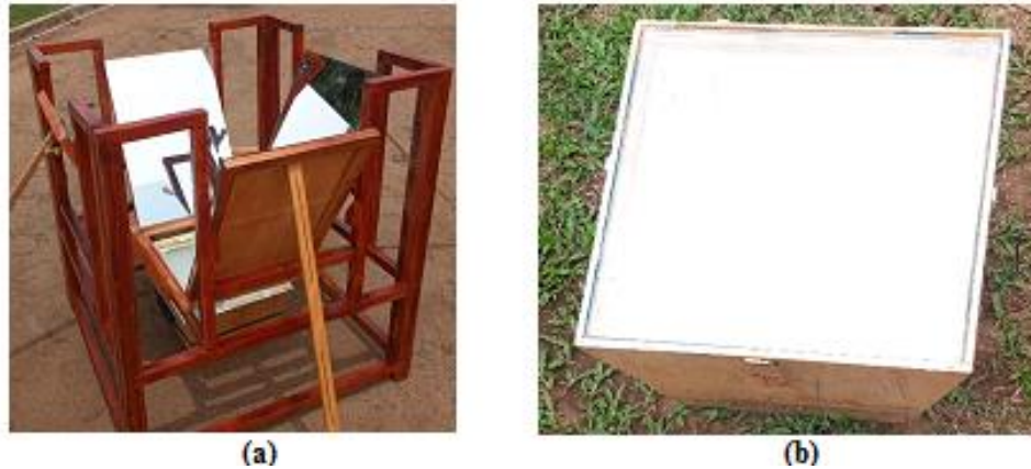
Figure 5: (a) Double V-trough solar concentrator (b) the truncated pyramid box solar cooker (Verma et al., 2022)
