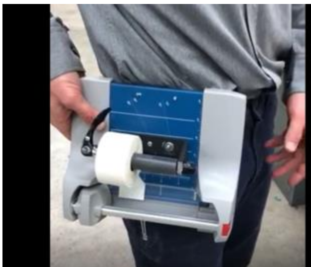
Figure 2. Athletic Tape Dispenser for one-armed operation
