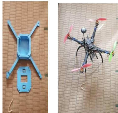
Figure 8: Drone Implementation, a) 3d Printed Drone's Frame; b) Drone prototype
