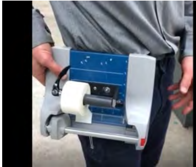
Figure 2. Athletic Tape Dispenser for one-armed operation
