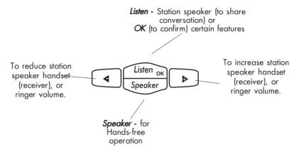
Fixed keys - horizontal and vertical Fixed keys correspond to frequently used features
