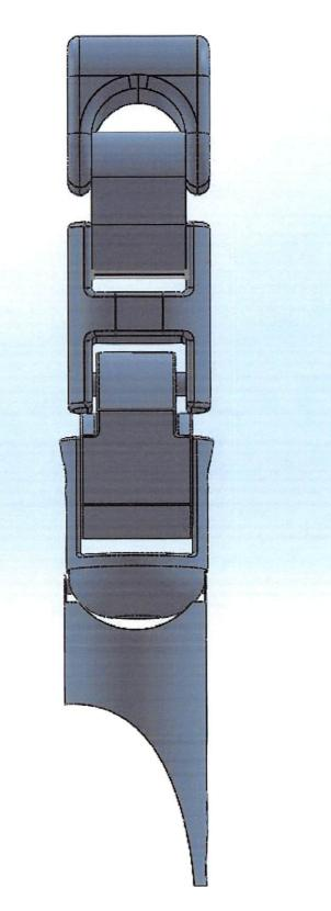
Figure - 4: Back View of a 3-D model of the proposed prosthetic finger
