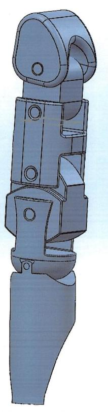
Figure - 1: Right-Side View of a 3-D model of the proposed prosthetic finger
