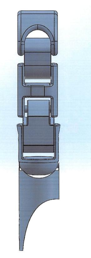
Figure -3: Front View of a 3-D model of the proposed prosthetic finger
