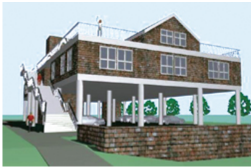
Tsunami resistant building with stilts
