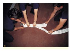
At this point, make another bend in the hose and return up to the 32-inch mark, continuing all the way around the top and back down the opposite side to a point just short of the male coupling. Once again, to keep the hose pack as compact as possible, don't go past the coupling.
