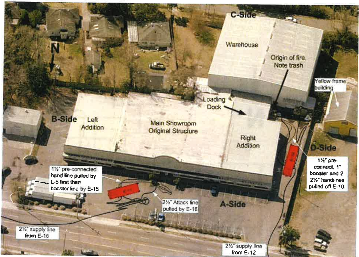
Diagram 2. Location of Engine 10 and Engine 11, supply lines and hoselines pulled at different times during the incident. Note accumulation of trash at loading dock on the day photo was taken, 3 months prior to the incident. Note the absence of ventilation ductworks or other roof penetrations over the showroom, thus no path for smoke and hot gases to escape. From aerial photo taken in March 2007 (copyright Pictometry International – used with permission of Pictometry)
