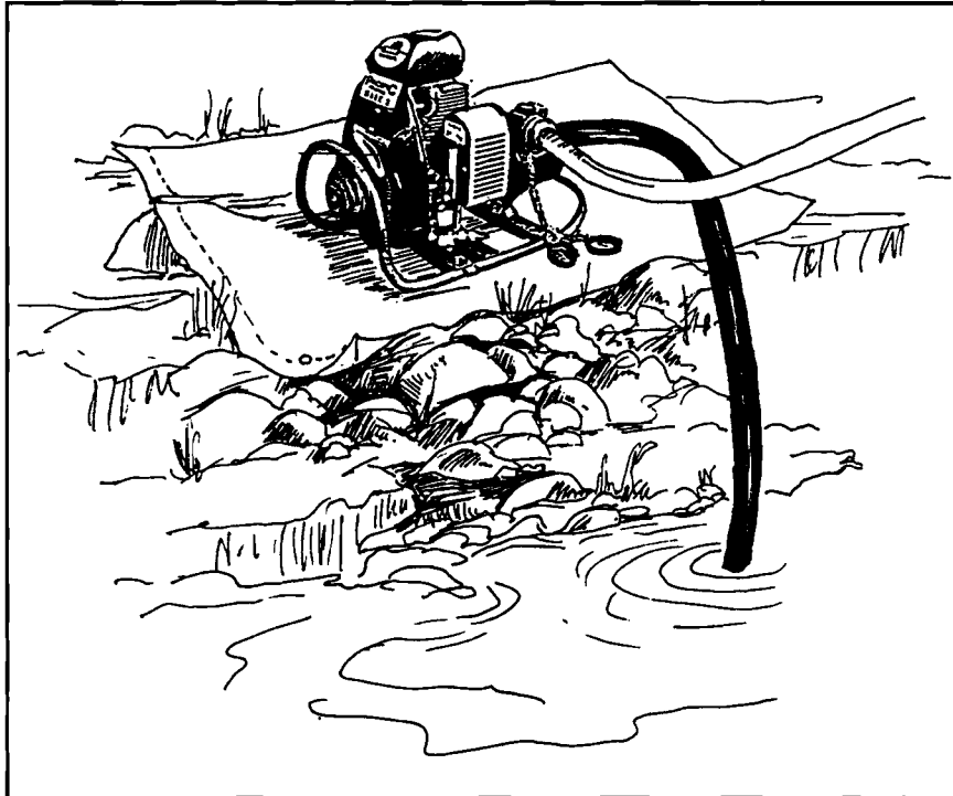
Figure 3—Set Up Pump Close To Water Supply
